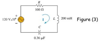
(Ans. a-  $\underline{w_s}$ =3727rad/s, Q=7.45, BW=500rad/s /// b-  $\underline{Pmax}$ =144W ///  $\underline{C}$ -  $\underline{w1}$ =3477rad/s ,  $\underline{w2}$ =3985rad/s )
