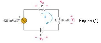
(Ans. a-  $R=25\Omega$ , C=4.05nF /// b- P=15.6mW /// c-  $V_c=39.3\angle-90$  ,  $V_L=39.3\angle90$  ,  $V_R=0.625\angle0$  )
